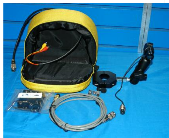
▲ The basic Catchit cam consists of a camera and mount, battery holder, wires, and a shock-proof bag to hold a video recorder. The system produces broadcast-quality images for about $600.
